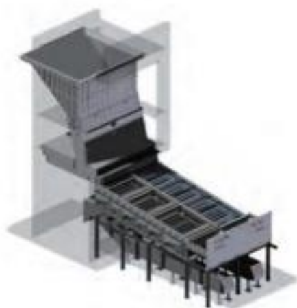
Waste to Energy Incinerator (Grate)
